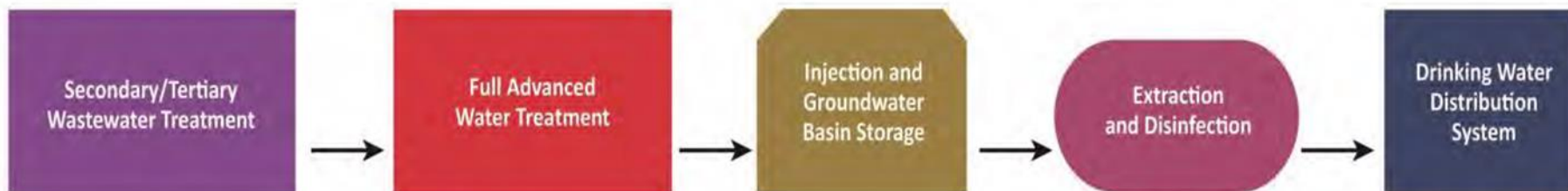
b) Indirect potable reuse using groundwater replenishment via subsurface injection .
